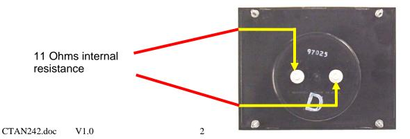
The value for a series resistor can be found using Kirchoff's voltage divider laws.
