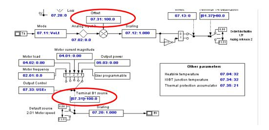
This resulted in the meter being slightly greater than full scale. This was corrected by utilizing the output scaling parameter. When the scaling parameter was decreased from 1.000 to 0.960, the voltage on the panel meter was reading full scale.
