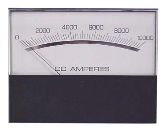
The analog outputs on our drives provide a nominal 10Vdc and can drive loads of approximately 5-10mA. Most commonly, panel meters require 50mV or 100mV to cause FS (full scale )deflection. Some meters will indicate FS = 1mA or 100uA. In any case, one must know at least one of these meter properties in order to interface properly.
